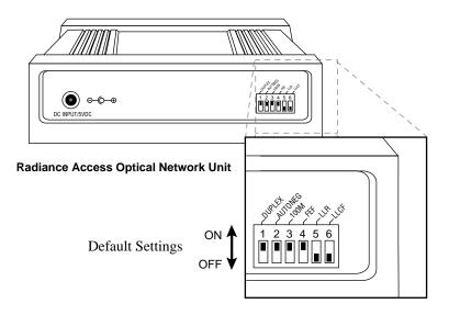
\* DIP switches can also be managed remotely via console commands or through Metrobility's NetBeacon or WebBeacon management software. Refer to the *Command Line Interface Reference Guide*, *NetBeacon Element Management Software Installation & User Guide* or *WebBeacon Management Software Installation & User Guide* for software management information.
